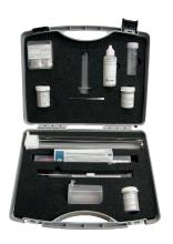
Hyprolyser® Test Kit contains all instruments, glassware and reagents to carry out all necessary routine and service tests to confirm and monitor the efficient operation of the system.
