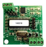
Modbus RTU module option available. Not included in standard scope of supply.
