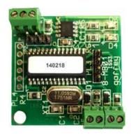
Modbus RTU module option available. Not included in standard scope of supply.
